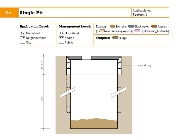
The single pit is one of the most widely used sanitation technologies. Excreta, along with anal cleansing materials (water or solids) are deposited into a pit. Lining the pit prevents it from collapsing and provides support to the superstructure.
